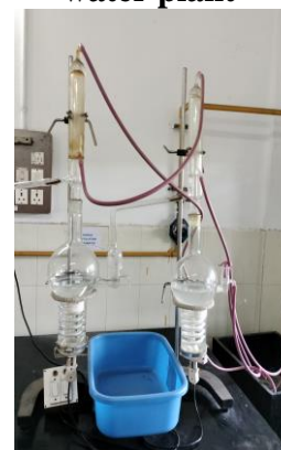
Double Distil water plant
